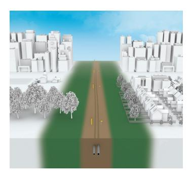
buildings and other structures. The corridor enables Pembina U.S. employees and contractors to access the pipeline for operations, inspections, maintenance, testing, and in the rare event of an emergency.
