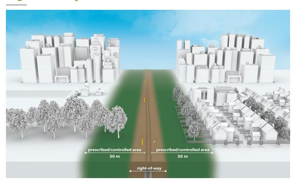
A pipeline right-of-way (ROW) is the strip of land where the pipeline is located, often recognizable because they are clear of trees, buildings and other structures. The area extending 30 meters (100 feet) on either side of the centerline of the pipeline is a safety zone (known as the Prescribed Area or Controlled Area).
