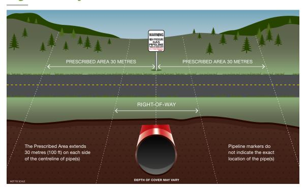
A pipeline right-of-way (ROW) is the strip of land where the pipeline is located, often recognizable because they are clear of trees, buildings and other structures. The area extending 30 meters (100 feet) on either side of the centerline of the pipeline is a safety zone (known as the Prescribed Area or Controlled Area).
